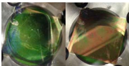
Figure 8. Photograph of an etalon in gasoline (left) before and (right) after addition of ethanol to gasoline to bring the concentration up to 12%. [Color figure can be viewed in the online issue, which is available at wileyonlinelibrary.com .]
